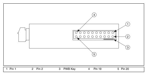
Figure 8. SCC Module Bottom View
